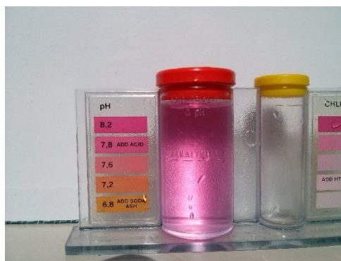
Calculating the acidity of a sample of water using a colour test and a constant background
