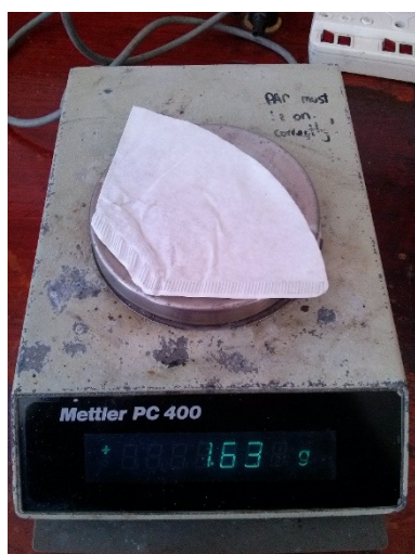
Weighing the sediment which has been left to dry in the filter paper
